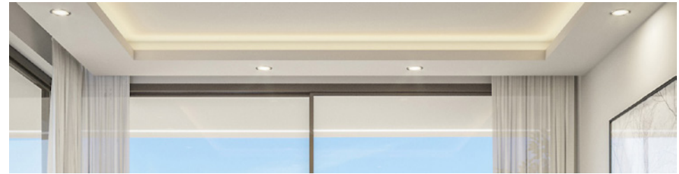
LED spot light & cove lighting
